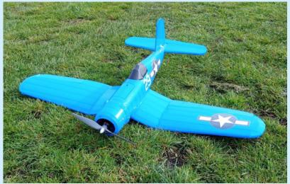
Our Spotlight Model this month is Derek's latest construction. It's a Corsair, built from a Flite Test free plan using the ever popular B&Q 6mm Extuded Polystyrene sheet. In this case the foam sheet was cold rolled to form the shape and, as Derek says, it was his hardest build yet. It also used more hot glue than he had ever used before. However, this and the blue packing tape used to cover it, helped keep the airframe
