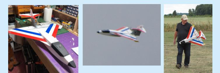
The Spotlight model for this month is Jon's Polaris. The first Polaris Club Build model to be finished and flown. With additional features such as the battery hatch opening device and the 'reinforced' motor pod. Jon has used a combination of coloured tape and paint to complete the colour scheme. Also, as the rear fuselage bottom is only taped on, the servos and receiver are still accessible.
