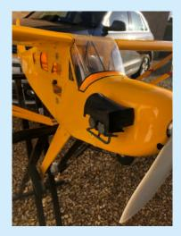
For the last of these, my own Volantex Ranger. Previously shown with the electronics out, it is now complete, and was flown on the 2nd December. The Eagle Tree Vector flight controller worked (it flew 'Home' when I threw the switch) but, with the C of G in the right place, it noses over on takeoff and landing. I've got three more weeks to try and modify the undercarriage!
