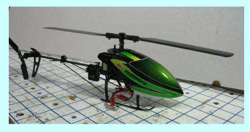
A diddy Spotlight Model this month. I'd been looking for a decent small helicopter for indoor flying, and found this at the BMFA Champs Swapmeet. It's a Walkera V120D025 and it came with a normal size, Devention Devo 7 transmitter, all for a modest £30. Within it's 12 inch rotor span it has
