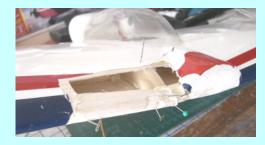
Just a couple of pictures of the Top Dawg during the repair, it now has a half inch thick rib forward of the spar.
