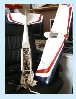
2. Checking the controls, the elevator moved the right way and the other controls moved. Note to self: (and reminder for others), don't just look for movement, check it's correct too. I'm publicising this embarrassing error of mine to, hopefully, prevent others from repeating it.
