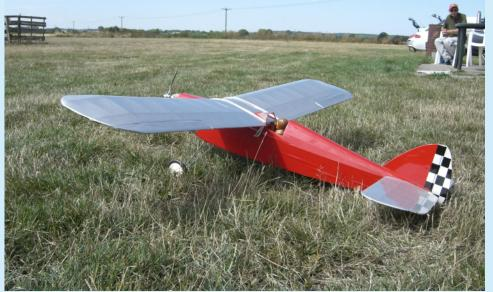
For the Spotlight Model this month, we have a 55" span Wifurskin that Steve Mason bought along to the field. Originally designed by J Bowmer in 1966, it was intended for 6 channel reed rc gear (rudder, elevator and engine, moving both ways) and a 0.19 cu in engine. The name is a combination of
